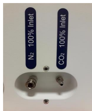
Figure 11.1 Gas inlets on the back of MIRI® and MIRI® Humidity multiroom IVF incubators
