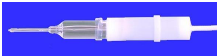
Figure 11.1 Micro pH probe for 0.5 \mu l drop measurement
