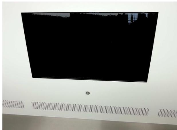
AIO PC with on/off button under the screen
