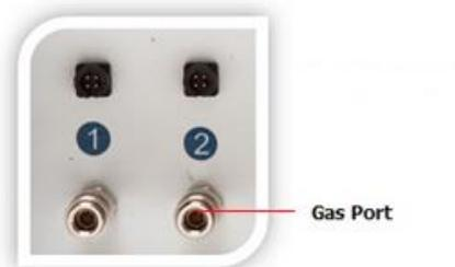
**Figure 24.1** Gas sample ports
