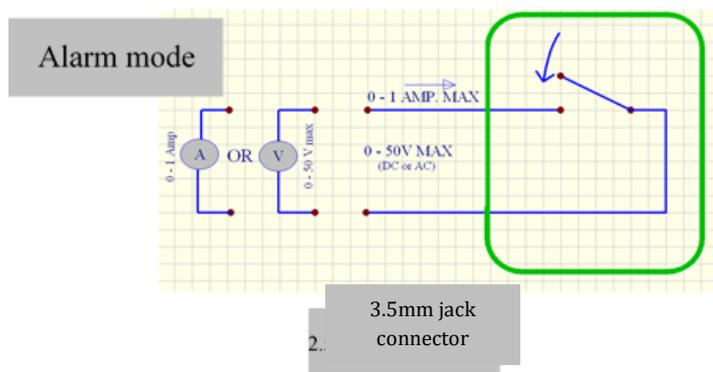
Figure 25.2 “Open circuit” alarm mode
