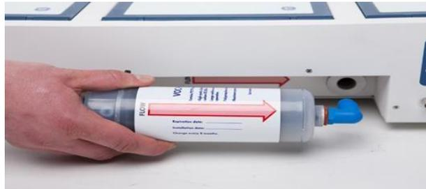
**Figure 11.2** The way of pulling the filter
