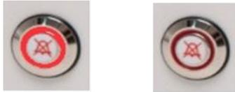
**Figure 14.1** Alarm key which indicates the alarm condition
