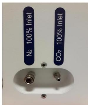
Figure 11.1 Gas inlets on the back of MIRI® Humidity multiroom IVF incubators
