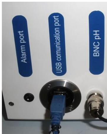
Figure 19.1 pH probe connected to the BNC
