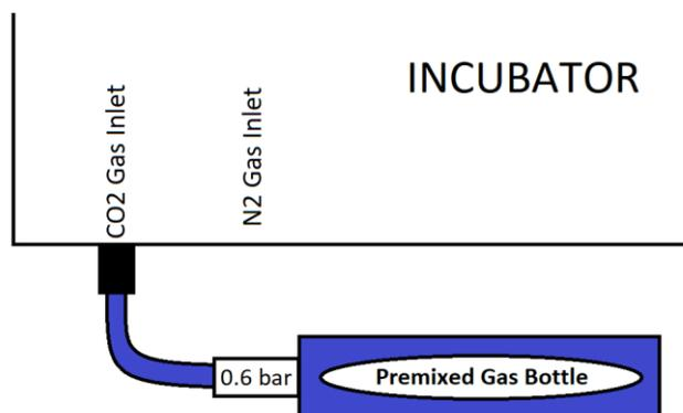
**Figure 13.1** Premixed gas connections to the incubator
