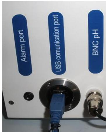
Figure 19.1 pH probe connected to the BNC
