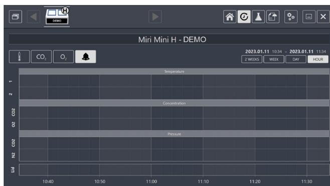
Conditions that put the Mini MIRI<sup>®</sup> Dry and Mini MIRI<sup>®</sup> Humidity into alarm state are recorded. It is possible for the software to send email alerts as well.
