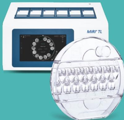
The lid is mounted inside the circumference of the dish covering the culture area completely – the user will only grab the dish during handling and not risk losing the dish by holding on to the lid only – as can be the case on all traditionally designed dishes. A large well is provided outside the culture area for pH measuring without affecting the cultured samples. The dish has a flat bottom so it is ideal for heat transfer from below.
