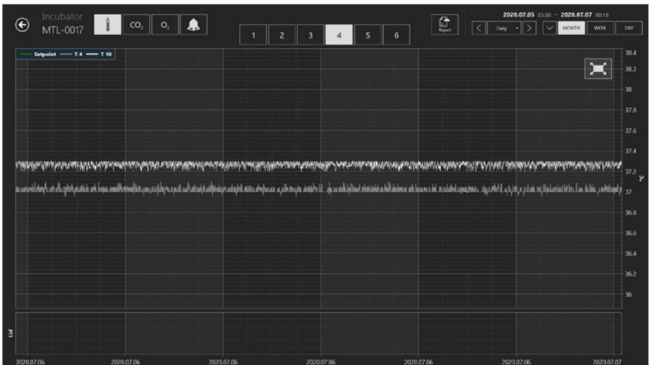
Conditions that put the MIRI® TL into alarm state are recorded. It is also possible to configure the software to send email alerts.
