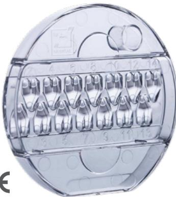
One (1) MIRI<sup>®</sup> TL chamber can hold one (1) CultureCoin<sup>®</sup>. Each dish can accommodate up to fourteen (14) embryos, each with a numbered well assignment. The MIRI<sup>®</sup> TL6 can hold up to 84 embryos, and the MIRI<sup>®</sup> TL12 up to 168 embryos.
